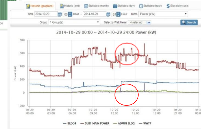
The peak demand power was caused by the power-on of the waste water treatment plant WWTP
